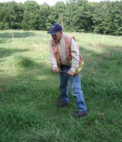
force has to come from the user. Also, unlike other probes if you run into a small rock, hardpan or other restrictive layer you can use the sledgehammer to find out what is truly solid bedrock without having to hire a backhoe, use your screw auger or dig a deep shovel hole.
